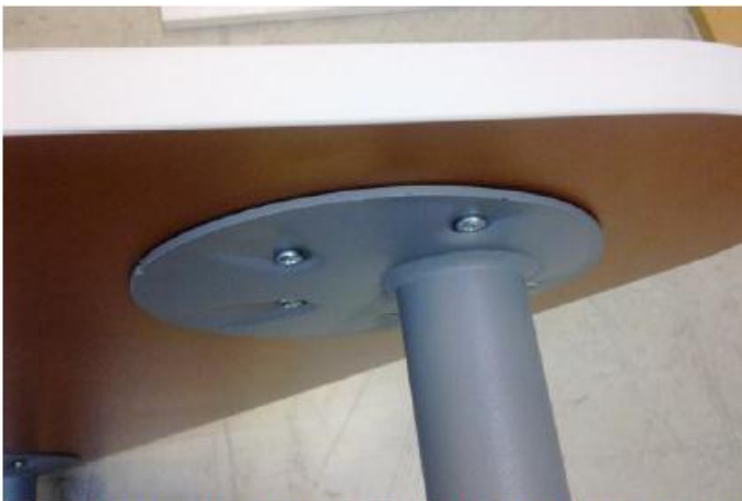
Picture 2: One screw loosened a bit during Horizontal fatigue test
